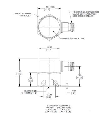
The Endevco® model 42A is a cost effective general purpose Isotron® accelerometer designed for use in a variety of applications. The model 42A is a small hex shaped Isotron accelerometer with a 10-32 side mounted connector. The unit is hermetically sealed against environmental contamination.
