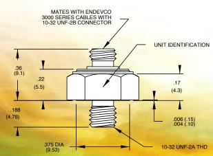
STANDARD TOLERANCE INCHES (MILLIMETERS) .XX = +/- .02 (.X = +/- .5) .XXX = +/- .010 (.XX = +/- .25)
