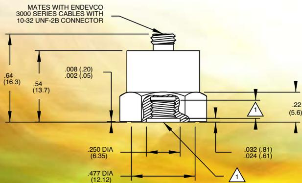
1 FOR MODEL 2225 (SHOWN), THREAD IS 10-32 UNF-2B, .125 MIN DEPTH.
